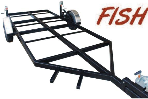
The image to the right is to illustrate the hitch assembly on these fish house frames. It is a crank down tongue. While the hitch is being cranked down, the receiver stays in the air and the rest of the frame lowers to the ice. This tongue also is equipped with a heavy duty crank jack and a coupler for a 2 inch ball.
