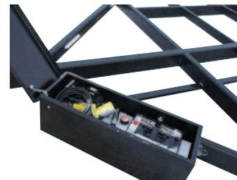
The image to the left shows the hydraulic pump used. Pump is powered by a 12V battery. Remote controlled.
