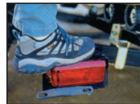
SUBMERSIBLE TAILLIGHT. Submersible waterproof taillights mount without brackets and double as steps.
