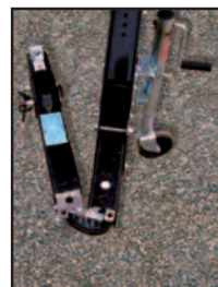
OPTIONAL SWING-AWAY TONGUE. Front portions of tongue swings away to shorten your trailer and maximize your garage space.
